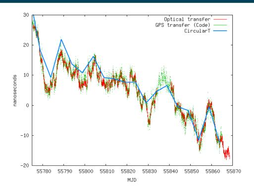
Red: time difference UTC(TP) – UTC(BEV) measured using optical link
