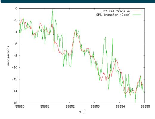
Red: optical transfer - linear regression over 780s Green: GPS CV
