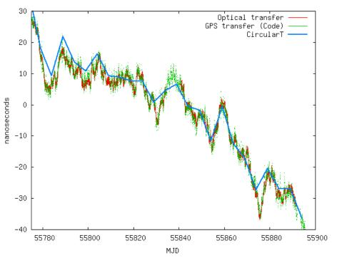
Red: optical time transfer Green: GPS CV Blue: Circular-T data http://www.bipm.org/jsp/en/kcdb\_data.jsp
