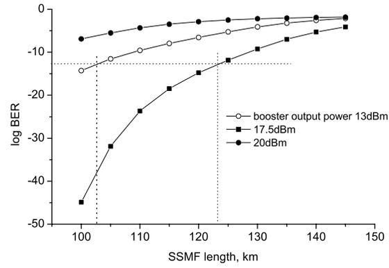
Fig. 3. Logarithm of BER as a function of SSMF length: no GVD compensation,  $P_{SSMF} = 13, 17.5,$  and  $20$  dBm.
