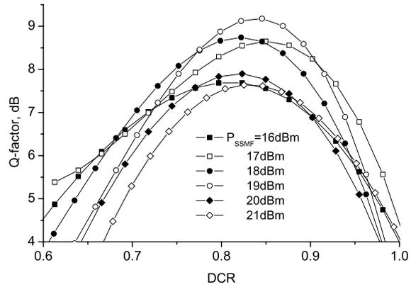
Fig. 6. Q-factor as a function of DCR for post-compensation scheme:  $L_{SSMF} = 270$  km,  $P_{SSMF} = 16, 17, 18, 19, 20,$  and  $21$  dBm,  $P_{DCF} = 0$  dBm.
