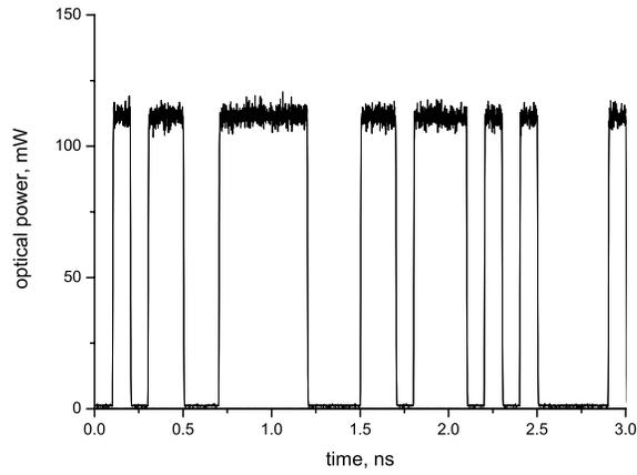
Fig. 4. Pulse shape at the input of 100 km of SSMF:  $P_{SSMF} = 17.5$  dB.
