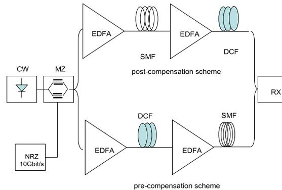
Fig. 1. Schematic diagram of post- and pre-compensation scheme under investigation.
