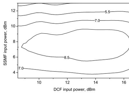
Fig. 15. Q factor as a function of  $P_{DCF}$  and  $P_{SSMF}$  for pre-compensation scheme:  $L_{SSMF} = 220$  km,  $L_{DCF} = 37.4$  km, ( $DCR = 0.85$ ).
