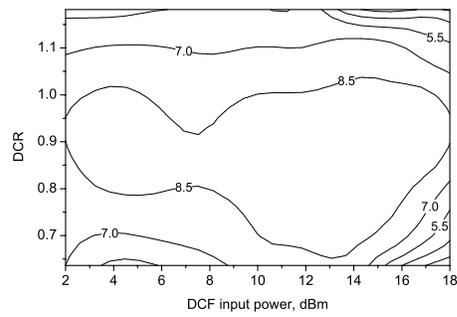
Fig. 13. Q factor as a function of  $P_{DCF}$  and  $DCR$  for pre-compensation scheme:  $L_{SSMF} = 220$  km,  $P_{SSMF} = 8$  dBm.
