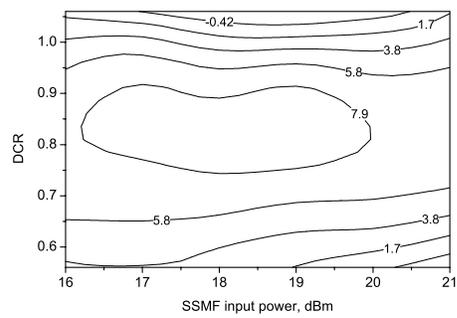
Fig. 7. Q-factor as a function of  $P_{SSMF}$  and  $DCR$  for post-compensation scheme:  $L_{SSMF} = 270$  km,  $P_{DCF} = 0$  dBm.
