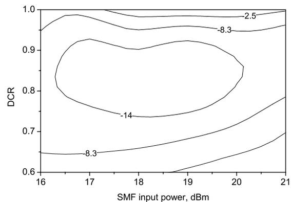
Fig. 8. Logarithm of BER as a function of  $P_{SSMF}$  and  $DCR$  for post-compensation scheme:  $L_{SSMF} = 270$  km,  $L_{DCF} = 45.9$  km, ( $DCR = 0.85$ ).
