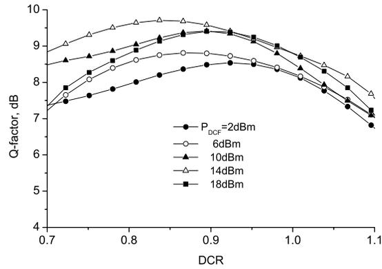
Fig. 12. Q factor as a function of  $DCR$  for pre-compensation scheme:  $L_{SSMF} = 220$  km,  $P_{SSMF} = 8$  dBm,  $P_{DCF} = 2, 6, 10, 14,$  and  $18$  dBm.
