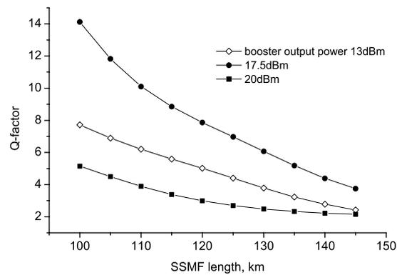
Fig. 2. Q-factor as a function of SSMF length: no GVD compensation,  $P_{SSMF} = 13, 17.5, \text{ and } 20 \text{ dBm}$ .
