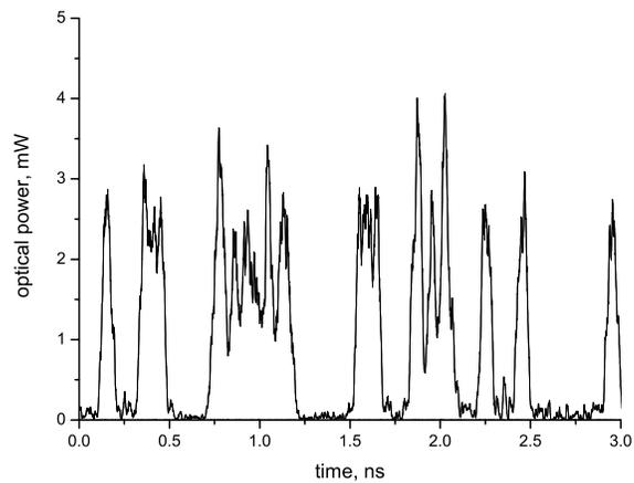
Fig. 5. Pulse shape after 100 km of SSMF: no GVD compensation,  $P_{SSMF} = 17.5$  dBm.
