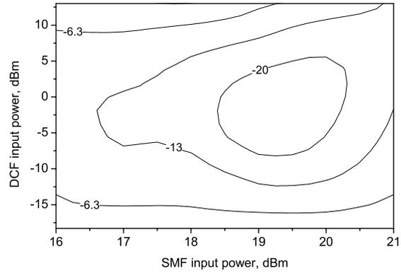
Fig. 10. Logarithm of BER as a function of  $P_{SSMF}$  and  $P_{DCF}$  for post-compensation scheme:  $L_{SSMF} = 270$  km,  $L_{DCF} = 45.9$  km, ( $DCR = 0.85$ )
