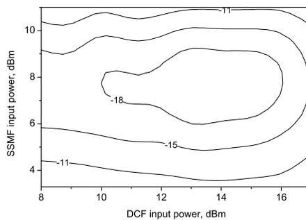
Fig. 14. Logarithm of BER as a function of  $P_{DCF}$  and  $P_{SSMF}$  for pre-compensation scheme:  $L_{SSMF} = 220$  km,  $L_{DCF} = 37.4$  km, ( $DCR = 0.85$ ).
