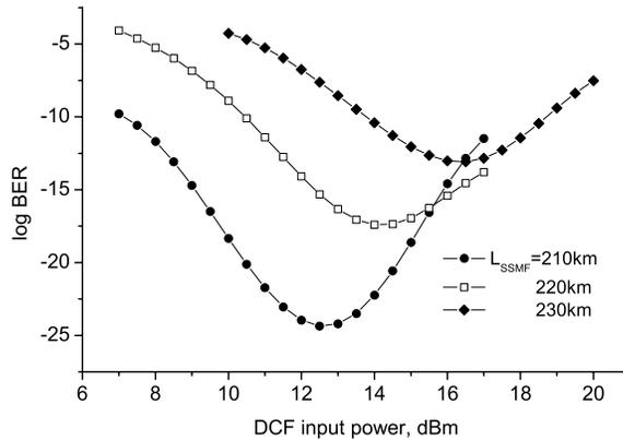
Fig. 11. Logarithm of BER as a function of  $P_{DCF}$  for pre-compensation scheme:  $L_{SSMF} = 210, 220,$  and  $230$  km,  $P_{SSMF} = 14$  dBm,  $DCR = 1.0$ .
