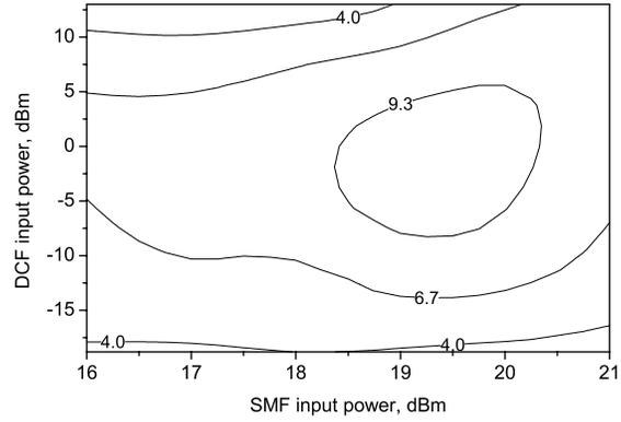
Fig. 9. Q-factor as a function of  $P_{SSMF}$  and  $P_{DCF}$  for post-compensation scheme:  $L_{SSMF} = 270$  km,  $L_{DCF} = 45.9$  km, ( $DCR = 0.85$ ).
