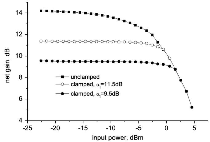
Fig. 2. Experiment: Single-channel (1545 nm) net gain of LRFA<sub>1</sub> as a function of input signal power with and without AOGC. Total loop loss  $\alpha_l = 11.5$  and 9.5 dB.
