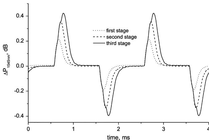
Fig. 11. Simulation: Output power variation of the 1545-nm signal at the output port of LRFA<sub>1</sub>, LRFA<sub>2</sub>, and LRFA<sub>3</sub> for the clamped cascade.  $\alpha_l = 10$  dB.
