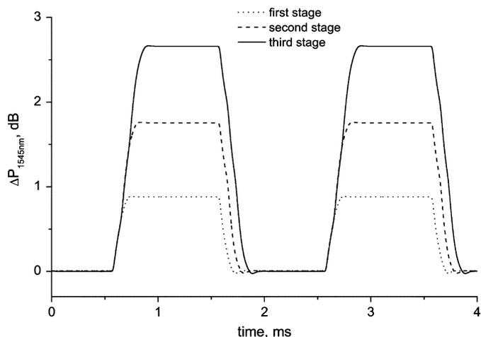
Fig. 10. Simulation: Output power variation of the 1545-nm signal at the output port of LRFA<sub>1</sub>, LRFA<sub>2</sub>, and LRFA<sub>3</sub> for the unclamped cascade.
