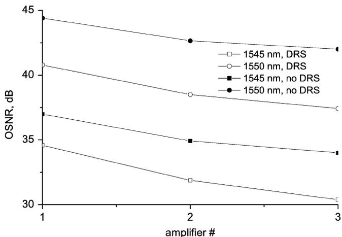
Fig. 9. Simulation: Evolution of OSNR along the cascade in case that the optical feedback loop of the LRFA<sub>1</sub> is closed ( $\alpha_l = 10$  dB) and the Rayleigh backscattering is taken into account or disregarded.
