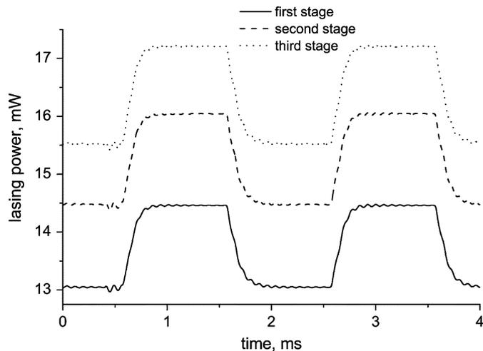
Fig. 12. Simulation: Time variation of lasing power at 1547 nm at the output of LRFA<sub>1</sub>, LRFA<sub>2</sub>, and LRFA<sub>3</sub>.  $\alpha_l = 10$  dB.
