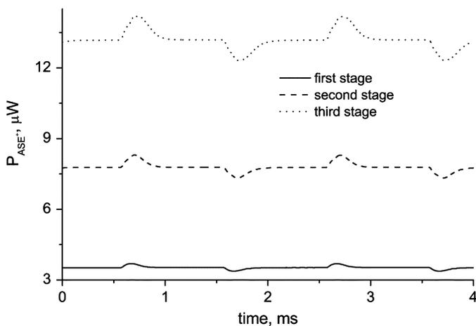
Fig. 13. Simulation: Time variation of downstream ASE power contained in a 1-nm slot centered at 1549 nm at the output of LRFA<sub>1</sub>, LRFA<sub>2</sub>, and LRFA<sub>3</sub>.  $\alpha_l = 10$  dB.
