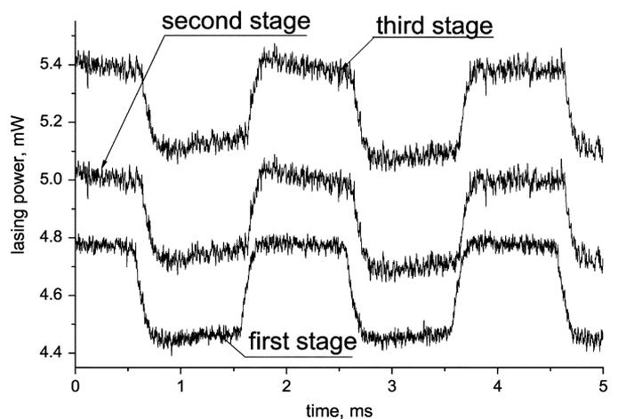
Fig. 6. Experiment: Time variation of the lasing power at 1547 nm recorded at the output of LRFA<sub>1</sub>, LRFA<sub>2</sub>, and LRFA<sub>3</sub>.
