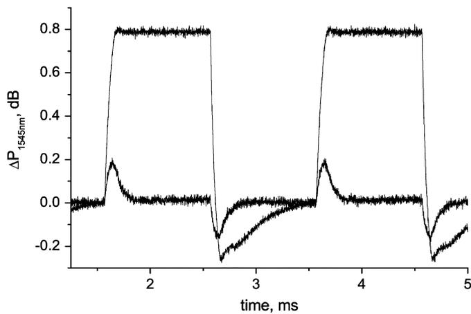
Fig. 4. Experiment: Output power variation of the 1545-nm signal at the output port of LRFA<sub>1</sub>: comparison of the unclamped and clamped regime.
