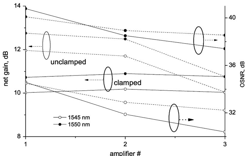
Fig. 8. Simulation: Net gain and OSNR of LRFA<sub>1</sub>, LRFA<sub>2</sub>, and LRFA<sub>3</sub> in the case in which the optical feedback loop of LRFA<sub>1</sub> is open and closed ( $\alpha_l = 10$  dB).
