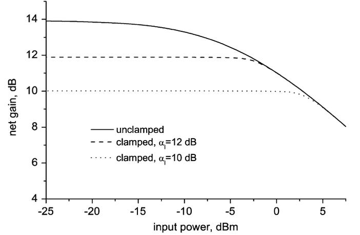
Fig. 7. Simulation: Single-channel (1545 nm) net gain of LRFA<sub>1</sub> as a function of the input signal power with and without AOGC. Loop loss:  $\alpha_l = 10$  and 12 dB.
