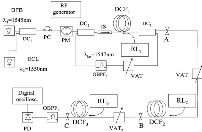
Fig. 1. Schematic diagram of the experimental setup of three AOGC LRFA's.
