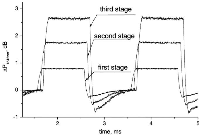
Fig. 3. Experiment: Output power variation of the 1545-nm signal at the output port of LRFA<sub>1</sub>, LRFA<sub>2</sub>, and LRFA<sub>3</sub> for the unclamped cascade.
