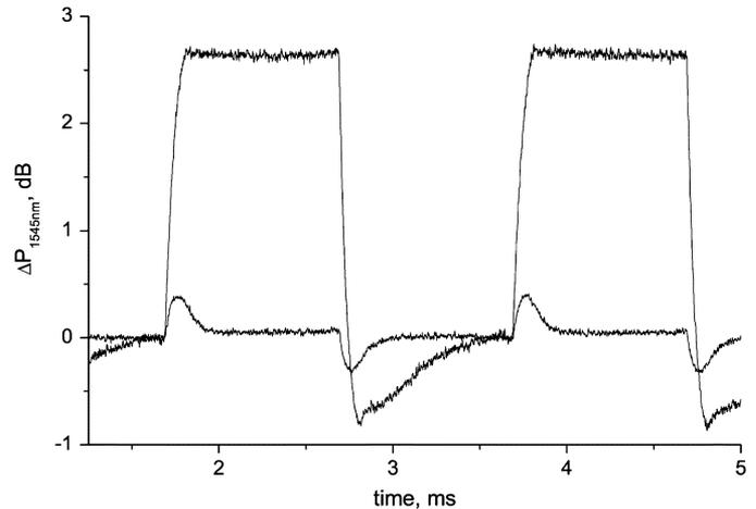
Fig. 5. Experiment: Output power variation of the 1545-nm signal at the output port of LRFA<sub>3</sub>. Comparison of the unclamped and clamped regime.
